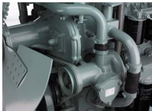
Fresh water pump
